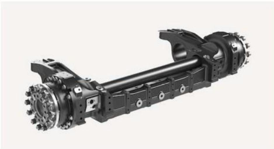
The cartridge assembly integrates the splined axle with the rotating part of the wheel that allows the wheels to turn. Each cartridge assembly includes 2 tapered roller bearing assemblies, and the whole assembly is held together tightly by a large locking nut (thrust nut), which is torqued at 3000 newton-metres of torque.<sup>2</sup> A cartridge assembly is installed on each end of a splined axle, secured with bolts.
