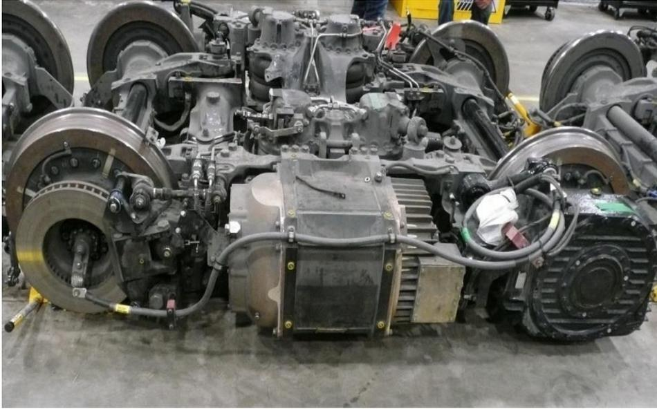
Among other components, each bogie is equipped with 4 resilient wheel assemblies and 2 axle assemblies. Each axle assembly includes 2 wheel hubs and 2 cartridge roller bearing sub-assemblies (cartridge assemblies) connected by a solid splined axle (Figure 3). The wheels are secured to the exterior of each hub by bolts to complete the bogie assembly. The axle transmits the weight of the vehicle to, and provides a smooth rolling movement for, the wheelset.
